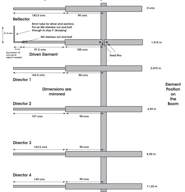
Antenna Model: 10/11M6 - 6 Element OP-DES Band(s): 11/10m 26.250-28.500 Elements: 6
