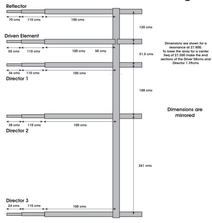
Antenna Model: 10M5/11M5 Heavy Duty OWA Band(s): 11 and 10m Elements: 5
