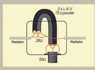
The basic principle is a quarter-wave line of two coax-cables in parallel. One end of the line ist connected to the radiator, the other to a socket, which is grounded at the metallic boom and has two functions:
