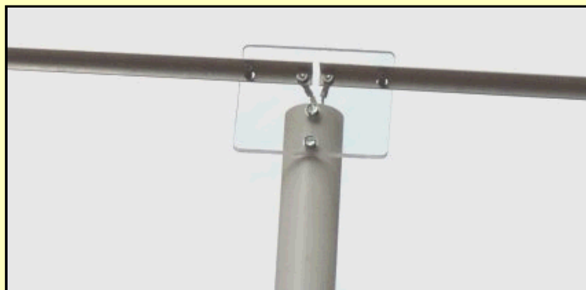
Photo C. The same assembly as in Photo B, but with an L-stock element--the outer support posts pass through holes in the element.
