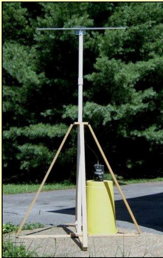
Photo A. The complete test assembly with a tubular dipole attached and the antenna analyzer stationed closer to the ground.
