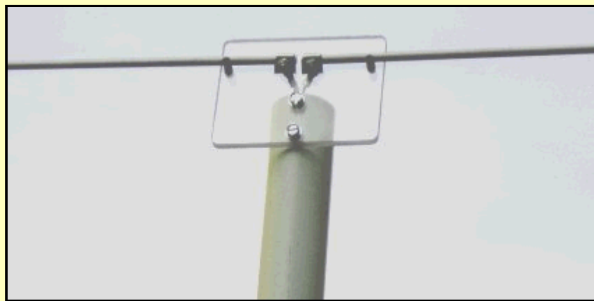
Photo B. A close-up of the center plate with a thin rod element clamped in place and supported by the outer posts.
