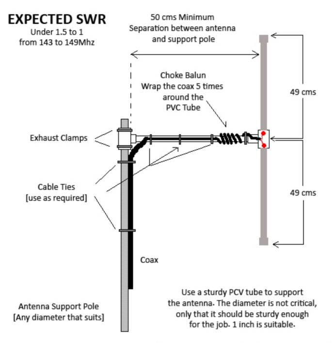
PVC tube to help keep the vertical parts of the antenna in some form of symetry [mainly when using wire] rather than aluminium tube
